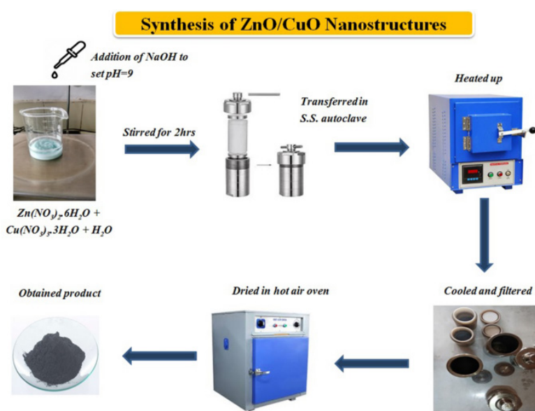
Figure 4. Hydrothermal synthesis of ZnO/CuO Nanostructures.
