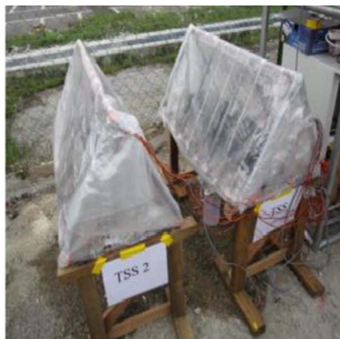
Figure 6. Single basin lengthy triangular solar still (Ahsan et al. , 2014).
