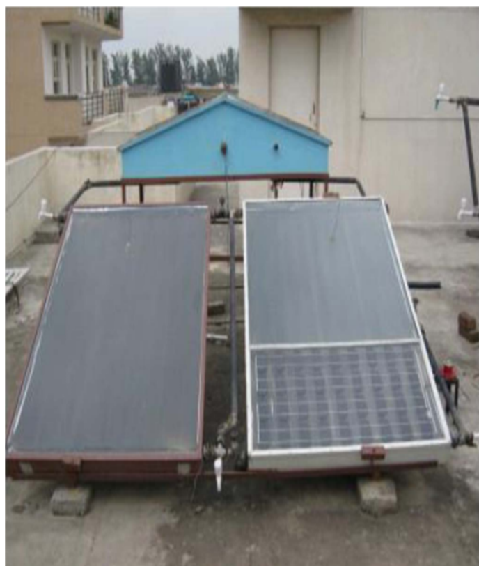
Figure 7. Single basin double slope hybrid solar still (Singh et al. , 2011).
