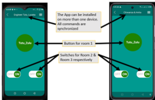
Figure 4. Switches and a push button used to control two bulbs Source: Author
