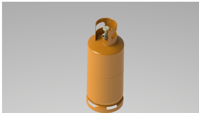
Figure 2. CAD modelling of CNG pressure vessel
