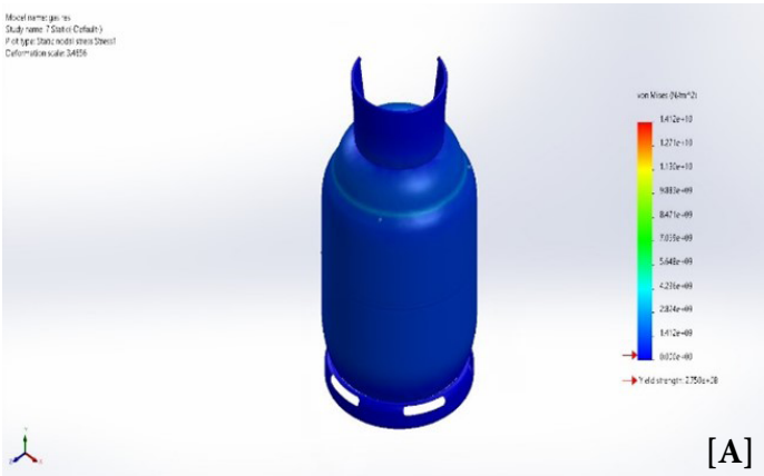
Figure 4. Static-stress analysis [A] Al 6061 material subjected to a pressure of 20 N/mm 2 and [B] 4130 steel material subjected to 25 N/mm 2 with a minor flaw
